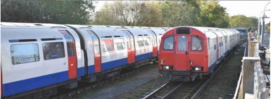
London Underground's Track Recording train consisting of 1973 ex Piccadilly Line carriage TRC666 (999666) sandwiched between 1960 Cravens driving cars L132 (97132) and L123 (97133) seen at Northfields, Osterley and Boston Manor on 15 November 2023. Paul Carpenter
