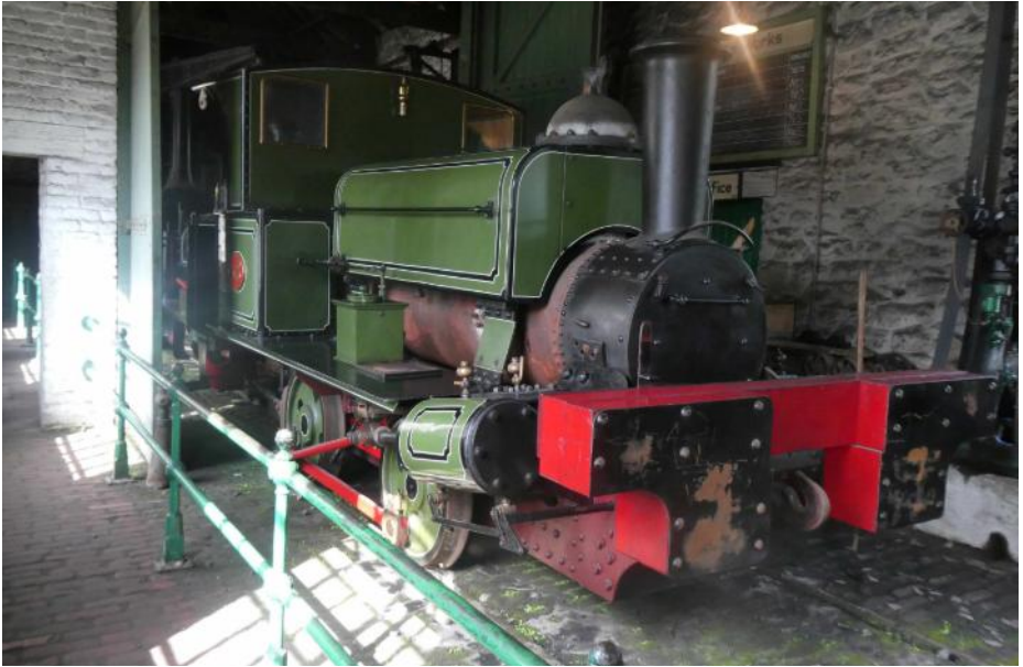
The famous 0-4-0ST No 18 built by Stephen Lewin of Poole in 1877 for the Seaham Harbour Dock Company.
