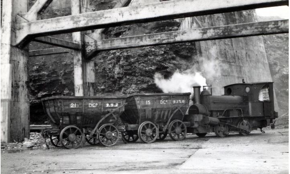
No.18 was used on the low level lines at Seaham Harbour (underneath the coal staithes) which were used for supplying coal and other provisions for use by the ship rather than cargo. Withdrawn around 1969 it's seen in this image working on 6 April 1963. WRS D318
