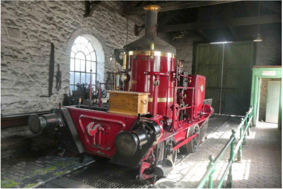
Former Betchworth Quarry Head Wrightson vertical boiler 0-4-0 of 1871
