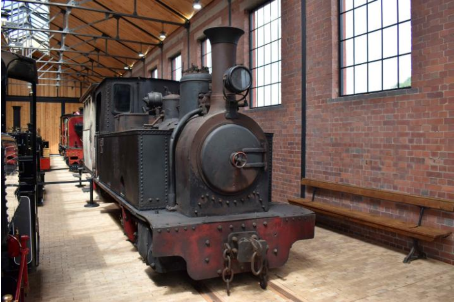
'Sabero No 1', built by Couillet in 1895, an 0-6-0T for the Hulleras de Sabero (colliery system) in Spain.
