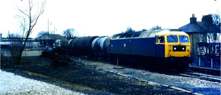
In January 1981 47118 shunts the oil tanks into the oil installation at Staines West, the curvature of the track showing that it wasn't the easiest place to shunt. 47118 has a silver painted roof, a trademark of Stratford depot, following the Silver Jubilee in 1977. 47114 - 47118 when built had a different Sulzer engine to standard, becoming Class 48 before being re-engined to conform with the rest of the class. In their standard Class 47 guise I worked on all this batch with the exception of 47118! Steve Guess
