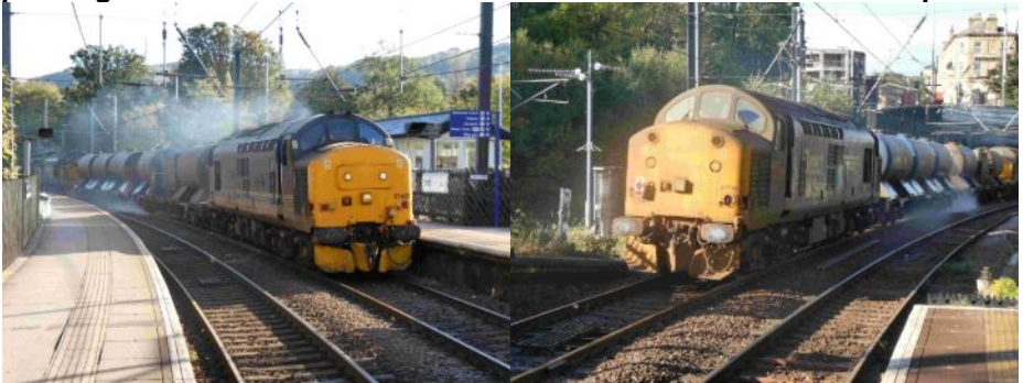
37425 and 37716 top and tail a rail head treatment train through Shipley station on 22 October 2023. Colin Aveyard
