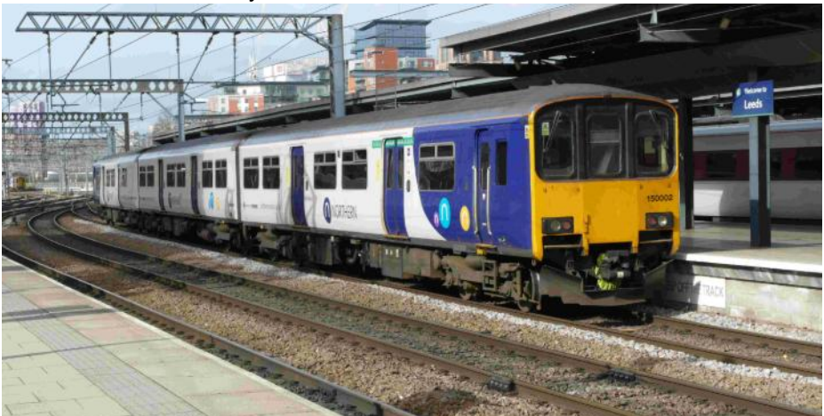
Northern Rail 150002 one of the two original three car Sprinter units is seen at Leeds station on 24 March 2023. Ken Aveyard
