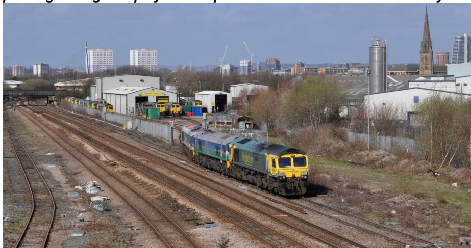
Class 59's under Freightliner now make regular appearances at Leeds Midland Road for tyre turning. Here 66418 backs 59002 and 59103 in to the depot on 22 March 2023. Howard Bolton
