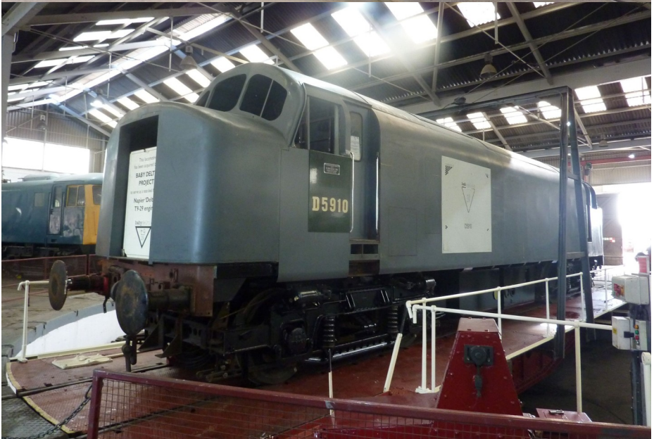
Little and large. D9009 Alycidon and D5910 the replica "Baby Deltic" being constructed from the shell of class 37 number 37372.
