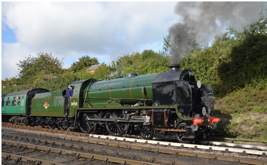
0925 Cheltenham which apparently struggled to gain traction on the Mid Hants gradients when running tender first. Plenty of sand was used!
