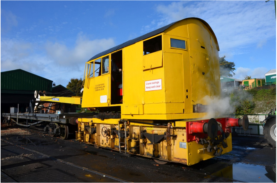
Ten ton crane DS58 built by Taylor and Hubberd of Leicester in 1955 and used at Woking Pre Assembly Depot.
