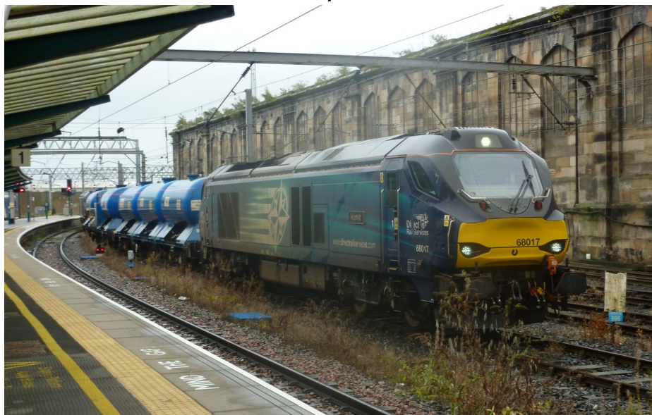
68017 at the head of a Rail Head Treatment Train, with sister loco 68001 bringing up the rear.
