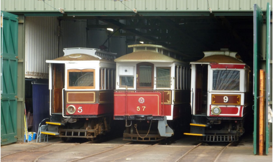
Manx Electric Railway trams at Derby Castle. Cars 5 and 9 are both Milnes cars of 1894 but to slightly different designs whereas car 57 is an enclosed trailer also by Milnes but from 1904. Colin Aveyard
