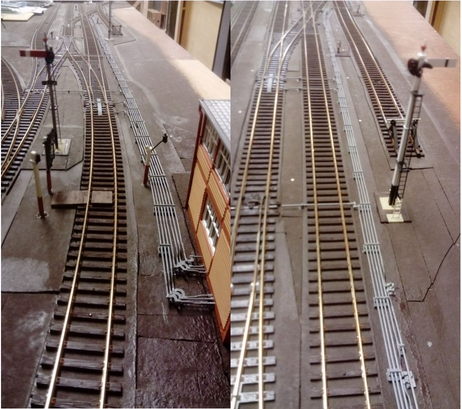
Left the start of the point rodding passing the single line token apparatus and right continuation of the run down to the single slip.
